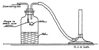
While the carbide is in position the gas is lighted and the air vents of the burner adjusted so the flame is barely non-luminous. The carbide is then shaken off into the water where acetylene is produced. The flame becomes quite luminous and remains so for a convenient length of time.
