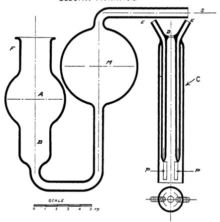
The apparatus is shown in the accompanying sketch and consists of an electrode holder, C, similar to an inverted test tube, containing the electrodes securely sealed in position; an opening at the top, D, to permit the introduction of a buret; the cell jar B expanded in the middle A into spherical form; a bulb, M, with a capacity approximately equal to the whole of the cell jar B and A.
